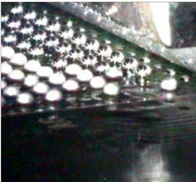
Fig. 3: Removal of residual solder in the process
